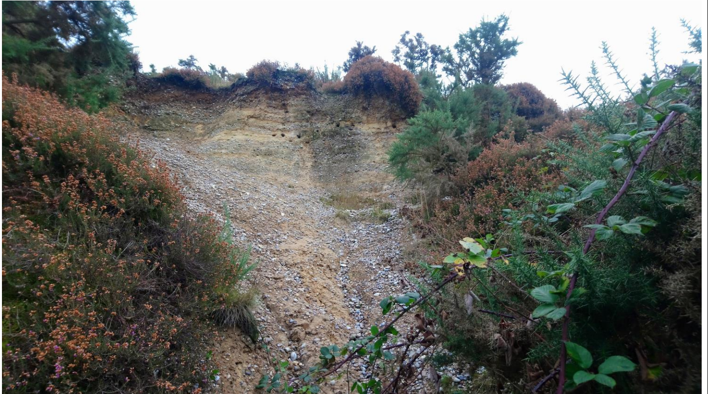
Photo 3 TM 44466845 looking south at the exposure in photo 2 - showing horizontally bedded sand and gravel. This is the face that was refreshed in 2015.
